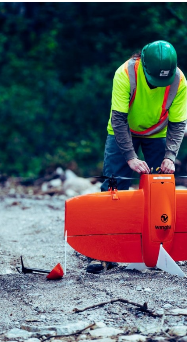
Vertical Takeoff and Land (VTOL) drone getting ready for flight. Photo credit: Rolute FP Canada Inc.
