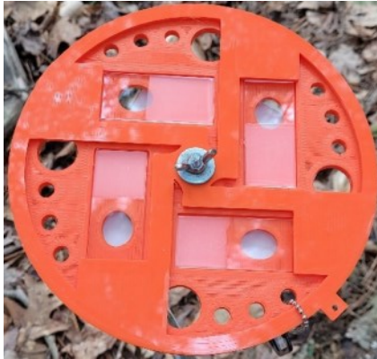
Novel 3D eDNA microscope slide traps for detecting hemlock woolly adelgid. Left: 3D printed trap. Right: Adelgid infested microscope slide. Photo credit: Natural Resources Canada.
